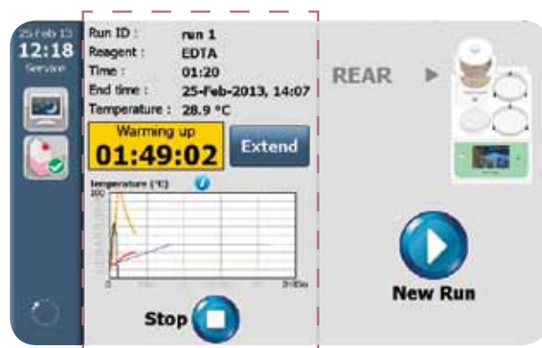
2 - Running a decalcification protocol with temperature curve
